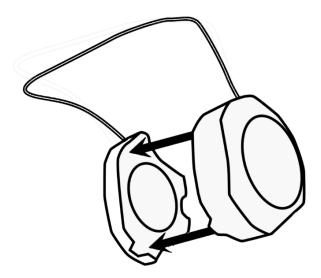
Hang the Spyder X2 unit over your display when asked, using the lens cap, which slides on the USB cable, as a counterweight to keep it in place. If necessary, angle your display back to keep the Spyder X2 flat against your screen.
