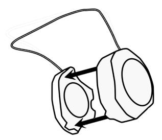
Hang the SpyderX unit over your display when asked, using the lens cap, which slides on the USB cable, as a counterweight to keep it in place. If necessary, angle your display back to keep the SpyderX flat against your screen.
