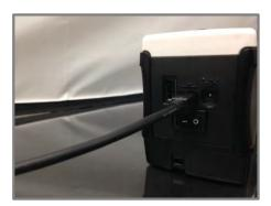
2. Connect the large USB connector on the instrument cable to a USB port on the computer.
