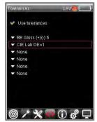
Press OK. The details of the tolerance are displayed, and the options on the Menu Bar change. The Editing options are displayed on the Live Bar:
