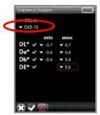
7. When you are finished, navigate to the Save Tolerance icon on the Live Bar and press **OK**.
