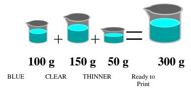
Starting with a known weight of a blue concennate, we add the minimum amount of resin needed to make it printable. In this case, 150 grams of clear vehicle are required. Next, we add enough solvent to bring the ink to our standard press-ready viscosity. In this case, it takes 50 grams of solvent. After mixing the press ready ink, we measure its density at 7.12 lb./gal.
