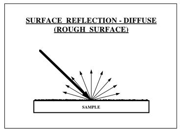
A matte sample - with a rough surface, the surface reflection occurs equally at all angles.
