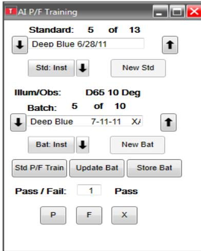
Another better option may be to add the pass, fail, exclude, and A.I. P/F training buttons to the ribbon bar (Shown below). The when searching for the button name they are 'Batch:P', 'Batch:F', 'Batch:X', and 'Standard:A.I P/F Training'
