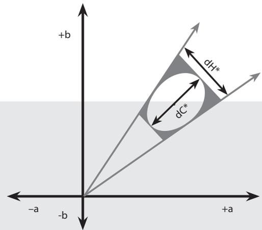
$$dE_{CMC} = \sqrt{\left(\frac{dL^*}{l S_L}\right)^2 + \left(\frac{dC^*}{c S_C}\right)^2 + \left(\frac{dH^*}{S_H}\right)^2}$$
