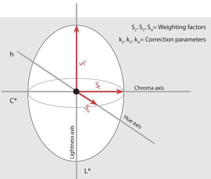
$$dE_{94} = \sqrt{\left(\frac{L_2^* - L_1^*}{k_L S_L}\right)^2 + \left(\frac{C_2^* - C_1^*}{k_C S_C}\right)^2 + \left(\frac{dH_{ab}^*}{k_H S_H}\right)^2}$$
