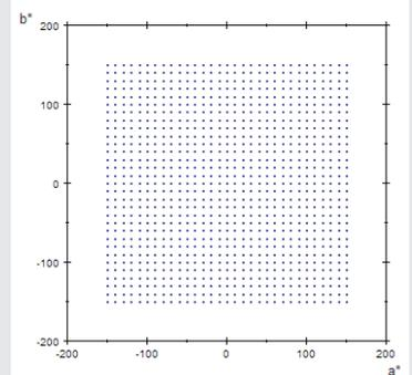
Step 1: rotation of the  $a^*/b^*$  plane by  $16^\circ$
