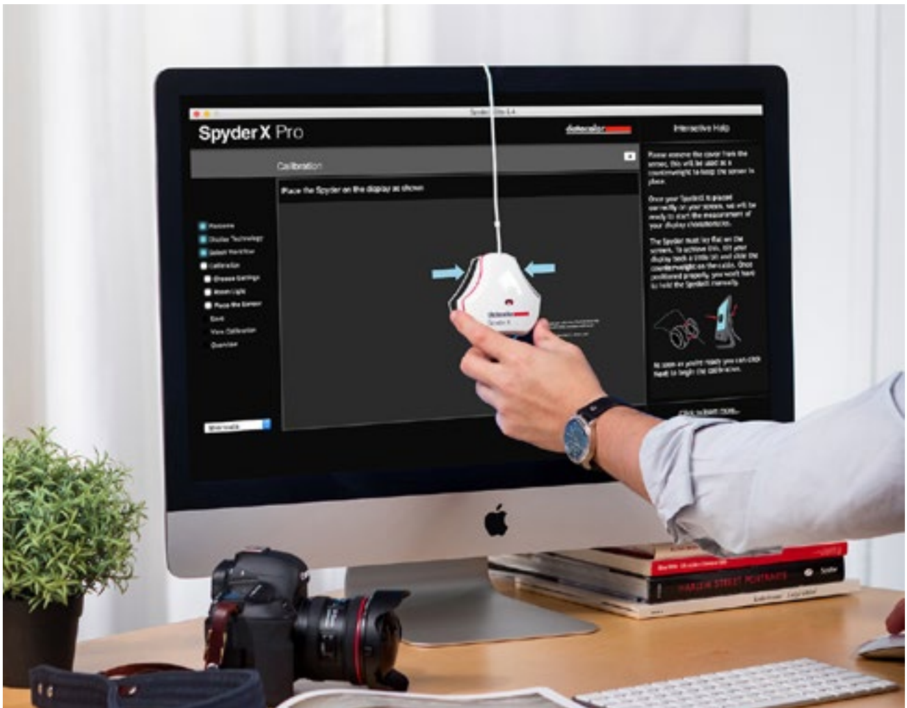
Hardware-based monitor calibration with a colorimeter.
